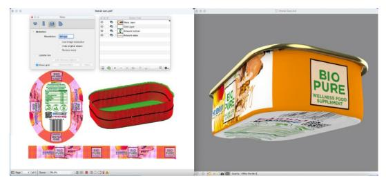
Capture 3D precise grid management with 2D and 3D mapping for accurate deformation and modeling in PACKZ.
